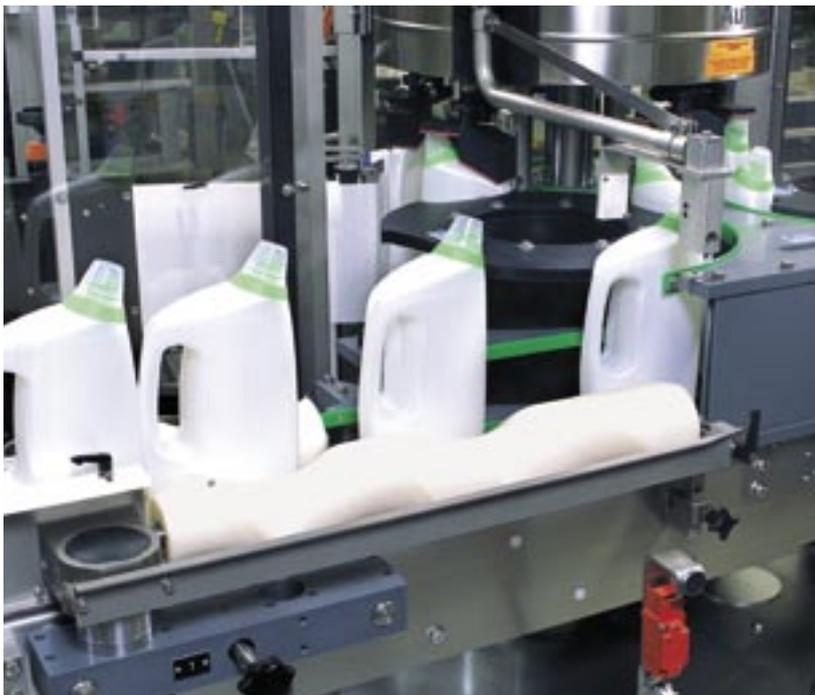
All models of the Autocol series can be quickly changed over to other container and label sizes without tools.
