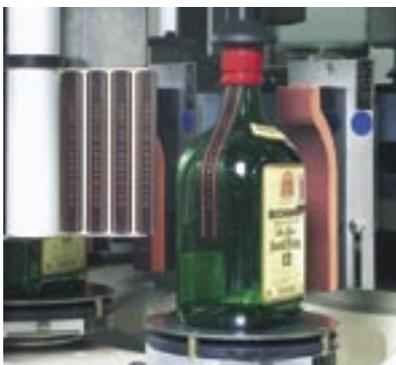
*Application of an additional self-adhesive label with cold-glue labeller*
