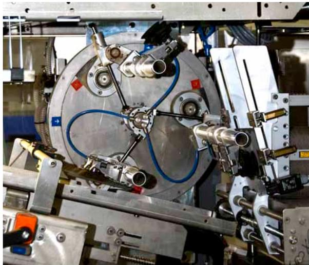
The carton blanks are below the container infeed. Vacuum grippers remove the first blank from the magazine and transfer it to the blanks feed. The secure separation and the conveyance of the carton blanks are performed via pivoting separators or roller separators and wide carton flights.
