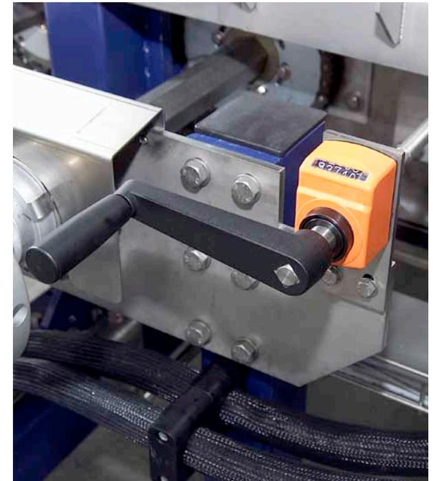
*Crank for infinite adjustments*
