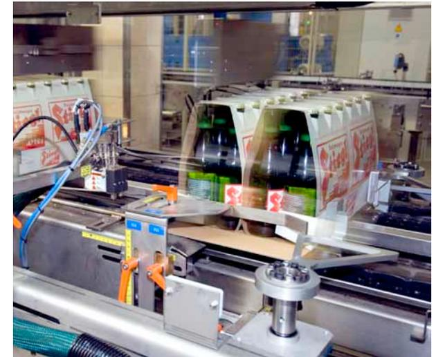
The shrink sleeve is fed air-supported so that the cutting module can process it without wrinkling. The conveyor in the film wrapping module and the compensation conveyor to the shrinking tunnel are equipped with an active conveyor centring unit and a rolling cutter edge. The precisely tempered hot air flow in the shrinking tunnel results in optimal shrinking. Thanks to the optimised temperature control with highly sensitive probes even thin film qualities can be processed without problems.
