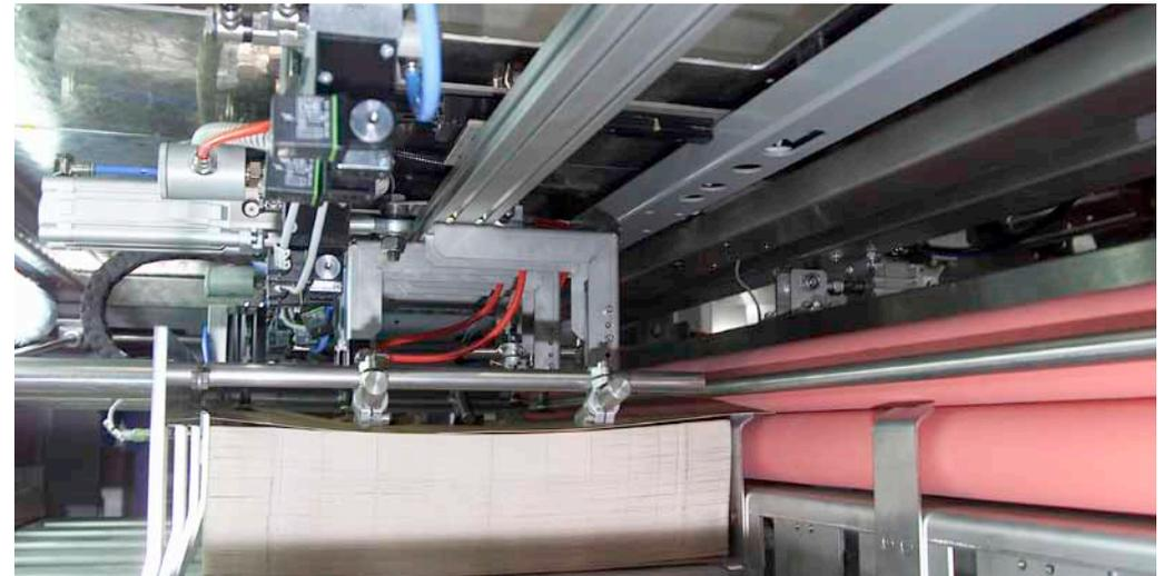
*Guide bars unfolding the carton.*
